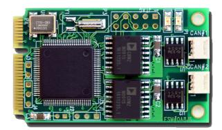
**MCAN-1020** is engineered around the ARM7 highly integrated microcontroller.
