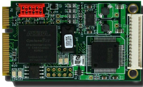
**MADC-1816** offers simultaneously sampling A/D architecture with 8 single-ended or 4 differential analog input channels. All channel features programmable gain 1 or 2 and can program to handle analog input with a single-ended or differential configuration.
